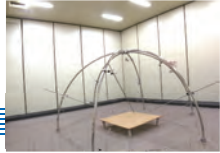
Measurement system for sound power level (NetdB system dB FA, dB Power)
